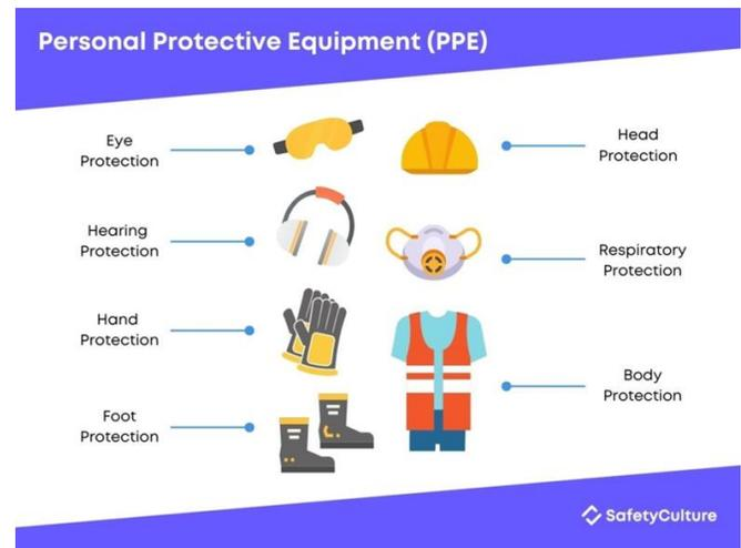
**Safety glasses** provide eye protection from flying chips, debris, and other eye hazards. Goggles protect your eyes from chemical splashes and face shields are a safeguard when worn over other protective eyewear, such as safety glasses.
